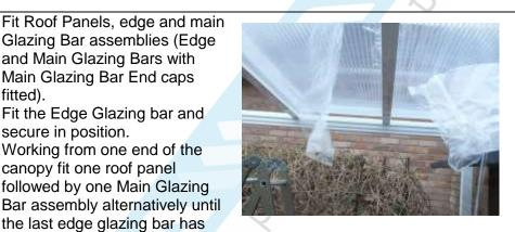
Position Main Glazing Bars -09 Check that the spacing between the Main Glazing Bars is correct. Mark these positions.
